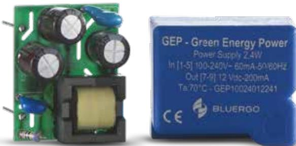
The GEP series is a line which is part of Bluergo's Le@f Brand. The GEP is a line of PCB Power supplies proposed as alternative to the traditional laminated transformers with many advantages: standard dimension if compared with traditional transformers, high efficiency, high power density. This matched together with its functional characteristics, with extended supply tensions guarantee favourable characteristics for every kind of application, from domestic to industrial.
